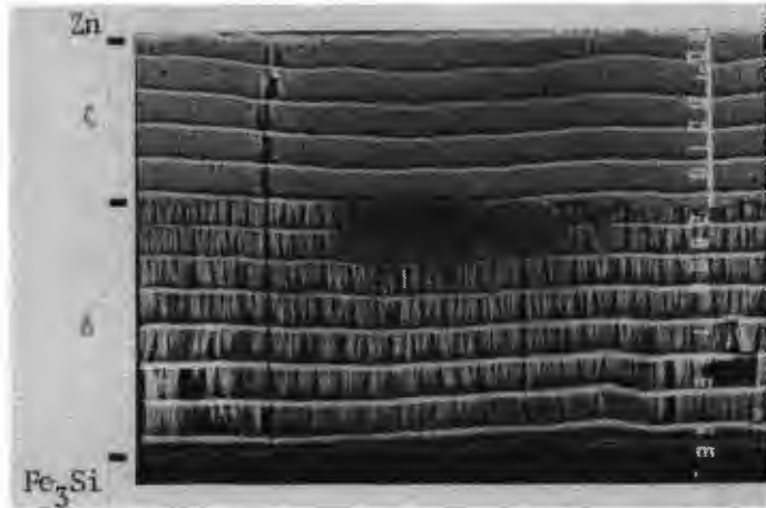
Fig. 5.34. Fe 3 Si-Zn couple, 24h, 395°C. Notice the periodic arrangement of thin bands throughout the \delta and \zeta reaction layers. The holes between the grains of the \delta layer are due to a prolonged etching (BEI). The white bar indicates 100 \mu\text{m} .
