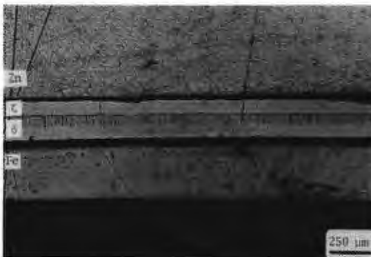
Fig. 5.53. Thin substrate Fe-Zn couple, 24h, 395°C. Notice the absence of cracks in the reaction layer.
