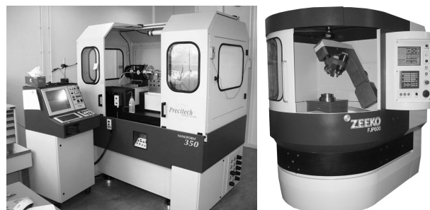
Figure 1: Free-form optics production facilities at TNO TPD
