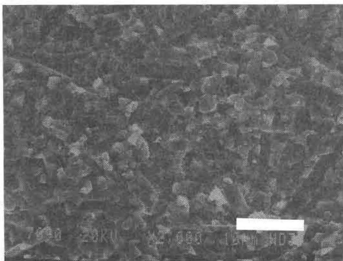
Fig. 5-21B: SEM micrograph of the fracture surface of \alpha'+\beta' -sialon (A4) with presintering at 1700°C, 90 min. The bar is 10 \mu\text{m} .
