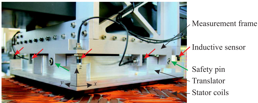
Figure 7.2. Detail of the measurement frame of the HPPA.
