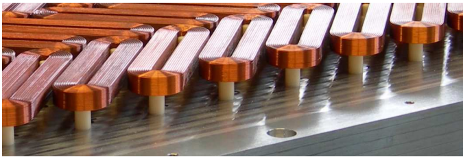
Figure 6.13. Coils in the planar actuator placed on aluminum oxide stands.
