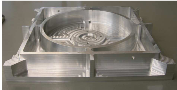
Figure 6.4. Stiff aluminum carrier.
