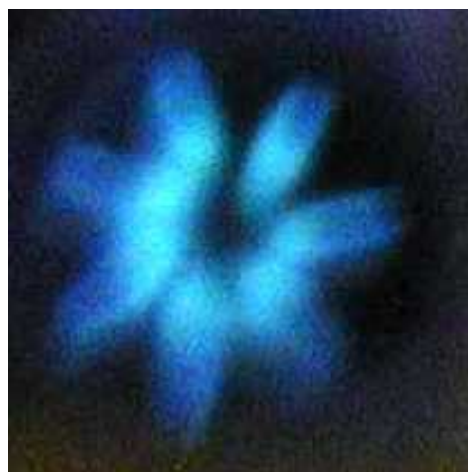
Figure 1.2 : Photograph of the 7 blue flames visible during the partial combustion process inside the micro-scale swirl-burner [39].
