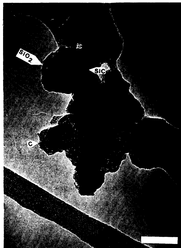
Fig. 3. TEM of a mixture of gas black, silica and SiC at 90% conversion. The length of the bar is 50 nm. The 35 nm spheres are gas black. The figure also shows submicron SiC particles which are covered with a layer of silica.
