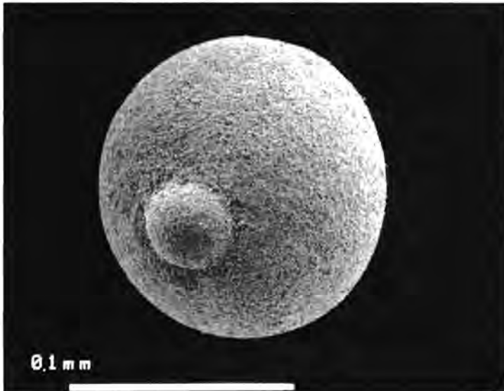
Fig. 4.14: Granule produced by spray-drying observed with SEM. Protruding from the granule is a smaller granule which has become attached during spray-drying. The presence of large agglomerates within the granule is not observed.
