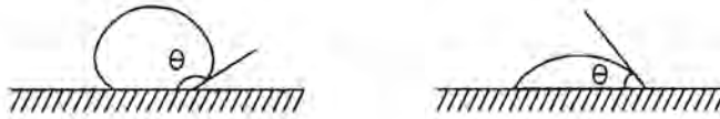
Fig. 2.1: Non-wetting property of mercury. With mercury, the contact angle \theta is larger than 90^\circ (left), whereas, with most liquids, \theta is smaller than 90^\circ (right).
