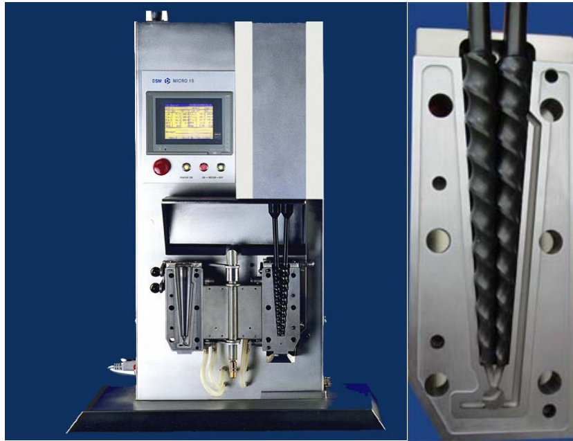
Figure 3.3: Picture of the DSM micro-compounder in which most of the chain extension work has been performed. On the left a view of the complete apparatus and on the right a close-up of the screws.
