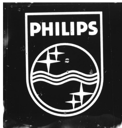
FIG. 6. Patterned LC layer between crossed polarizers. Philips logo.
