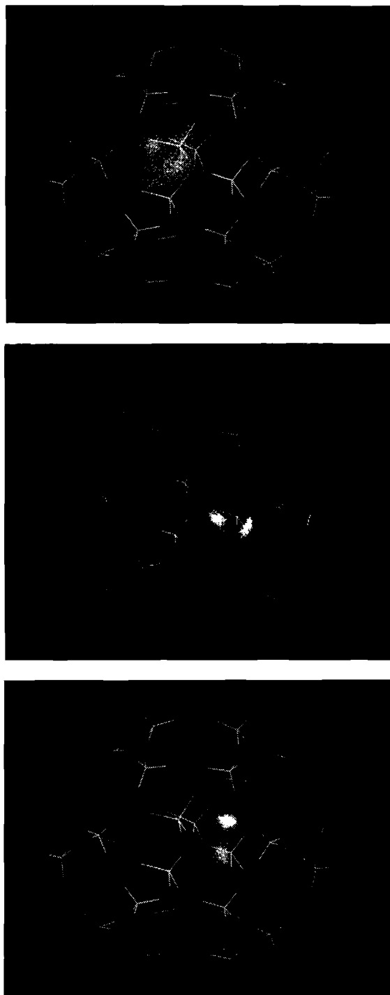
Figure IV.1 Rotational freedom of TMA occluded in the Sodalite \beta -cage at T=273 K (a), T=153 K (b), and T=123 K (c). The dots in the figures display the position of one TMA hydrogen atom at 50 fs time intervals.
