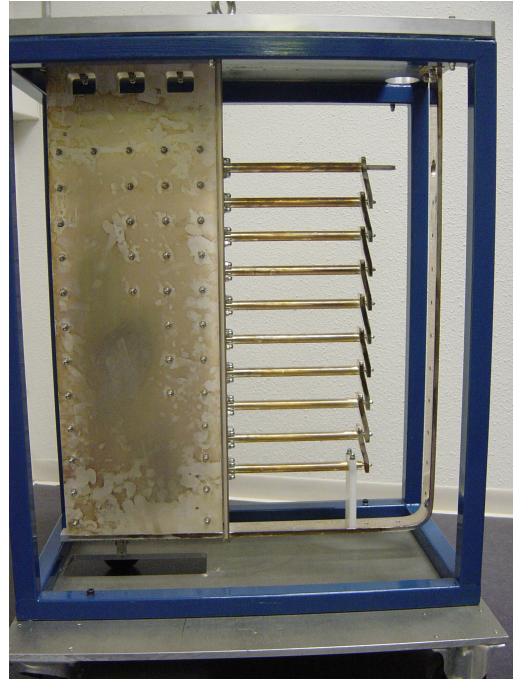
Fig. 6. Transmission line transformer; the dimensions are: 635 mm long, 734 mm high and 350 mm wide
