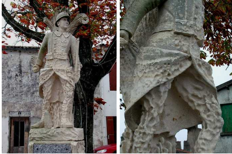
Figure 1.4: A statue of a soldier in La Rochelle (France). The legs of the statue have suffered erosion caused by salts. (Photo by Rob van Hees)
