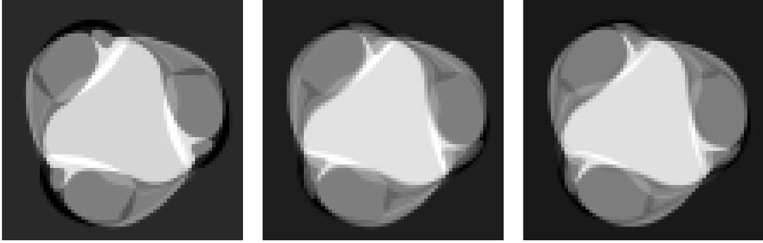
Figure 6.5: Here the temperature profiles are shown for an m = 3 perturbed equilibrium at t = 10.0\tau_A , where temperature jumps were applied at the original contours at r = R_1, R_2 . The left figure corresponds to a simulation with discretization level N = 3 , the middle for N = 5 and the right figure for N = 10 . Note that the middle figure corresponds to the contours shown in Fig. 6.4.
