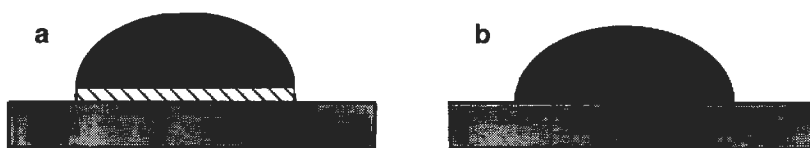
Figure 18 Schematic model of the metal-support interface after reduction at a) 300°C and b) 450°C.
