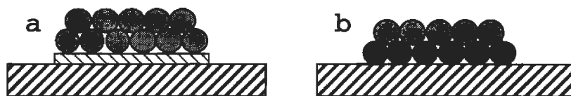
Figure 12 Schematic representation of the changes in the structure of the metal-support interface as a function of the reduction temperature. a) LTR: hydrogen present in the metal-support interface, b) HTR: interfacial platinum atoms in direct contact with support.
