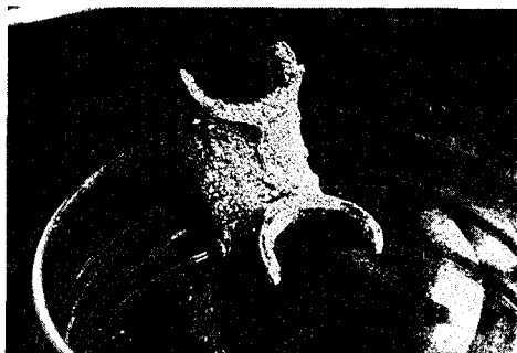
Fig. 14: A polypropylene-novalox saddle, fully grown with a dichloromethane degrading biofilm.
