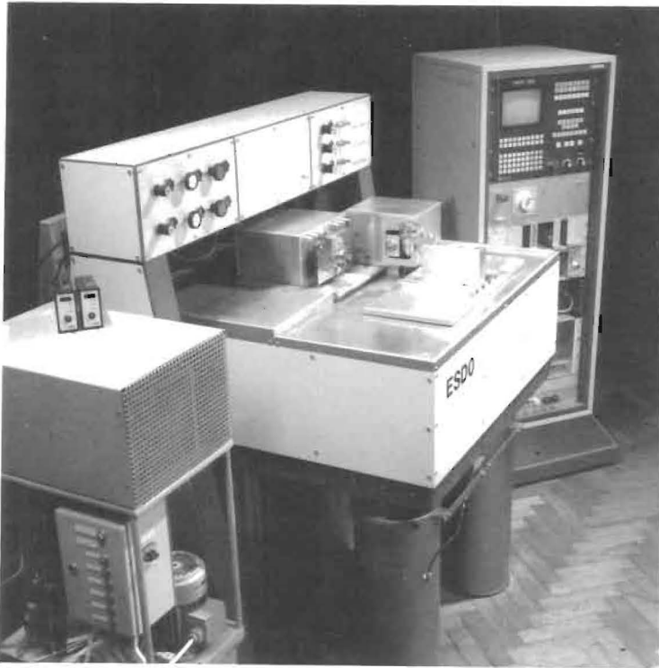
Fig. 1.8 The experimental diamond turning and grinding facility ESDO built as part of the research programme.
