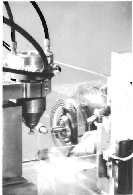
Fig. 1.7 Detail of the Kolatje, showing the specimen, the grinding spindle and the dress facility.
