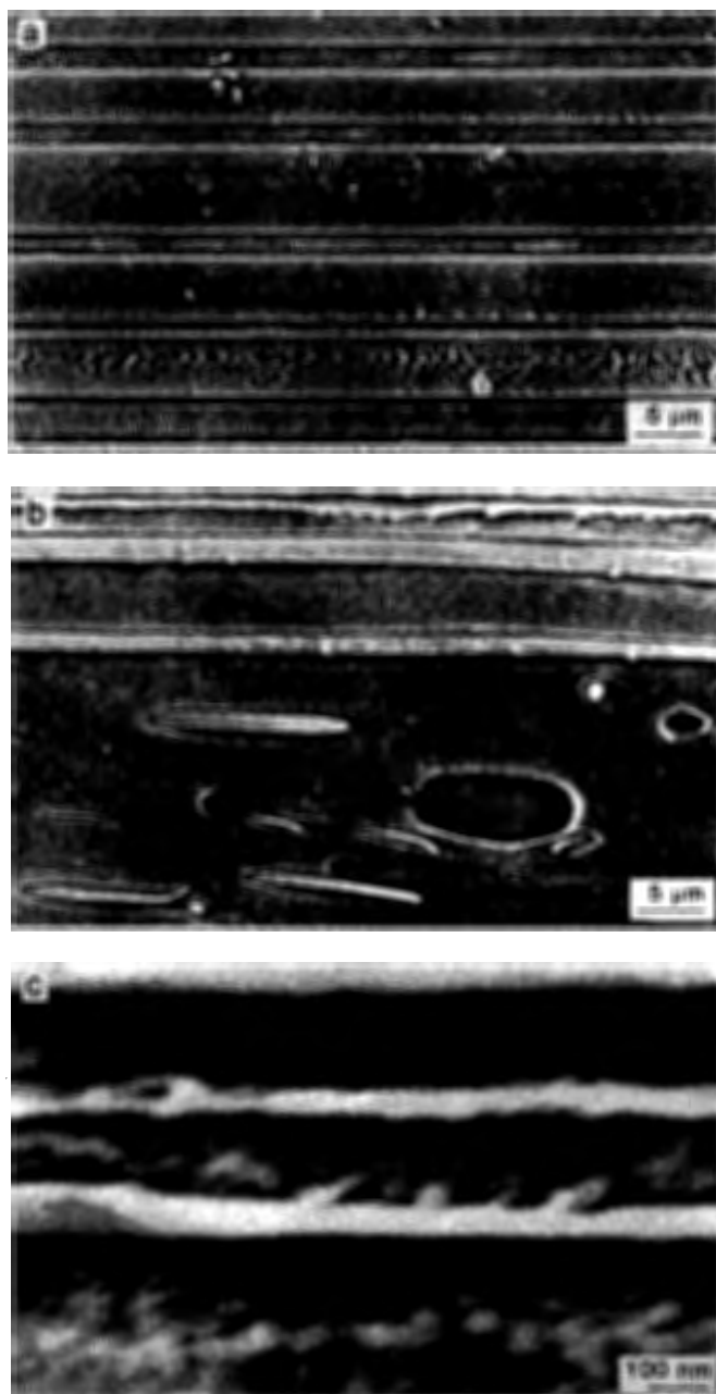
Figure 3.3 SEM micrographs of multilayered PS-PPE/PE tapes: (a) PS-PPE/PE 75/25 (PS-PPE 80-20), 6 mixing elements, (b) PS-PPE/PE 25/75 (PS-PPE 80-20), 11 mixing elements and (c) PS-PPE/PE 25/75 (PS-PPE 60-40), 11 mixing elements
