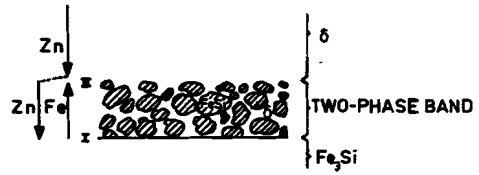
Fig. 5. Diffusion mechanism at Fe 3 Si substrate (see also text)
