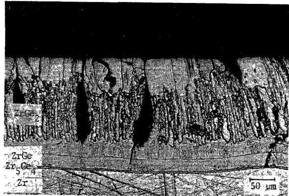
Fig. 7. Zr-ZrGe 2 diffusion couple annealed for 23 h at 1493 K.
