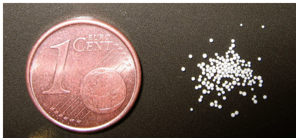
Figure 1.1 Novozym 435 is an immobilized preparation of CALB. The acrylic resin beads have a size of 0.3 – 1.0 mm and contain approximately 10 wt.% protein.
