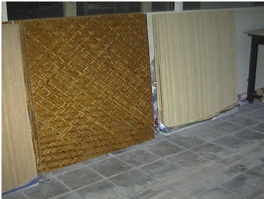
Figure 3. Bamboo mat boards (left) and bamboo strip boards (right).
