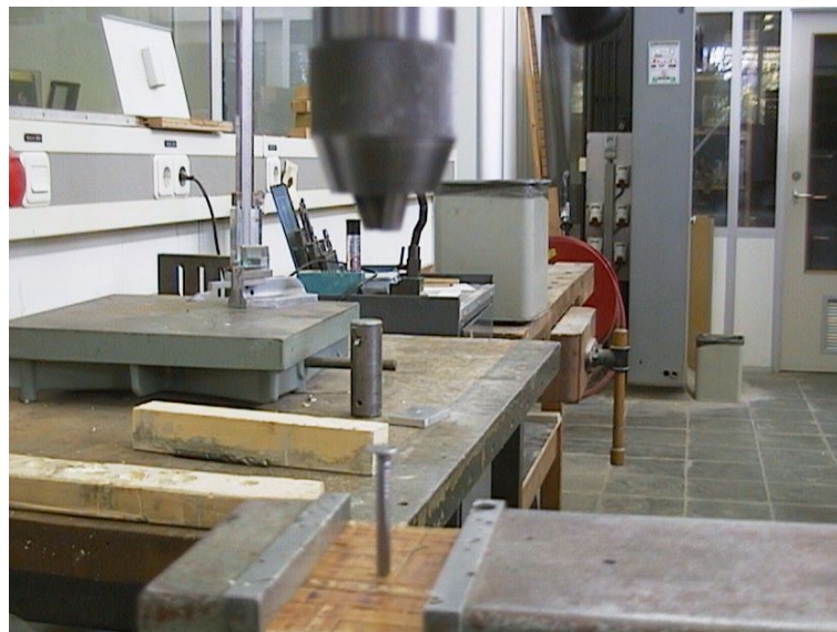
Figure 7. Placing the nail into the specimen.
