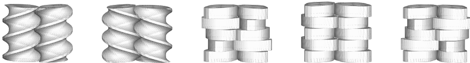
Fig. 5.1: Basic types of twin screw extruder elements. From left to right: conveying element, counter conveying element, conveying kneading section, neutral kneading section and counter conveying kneading section.
