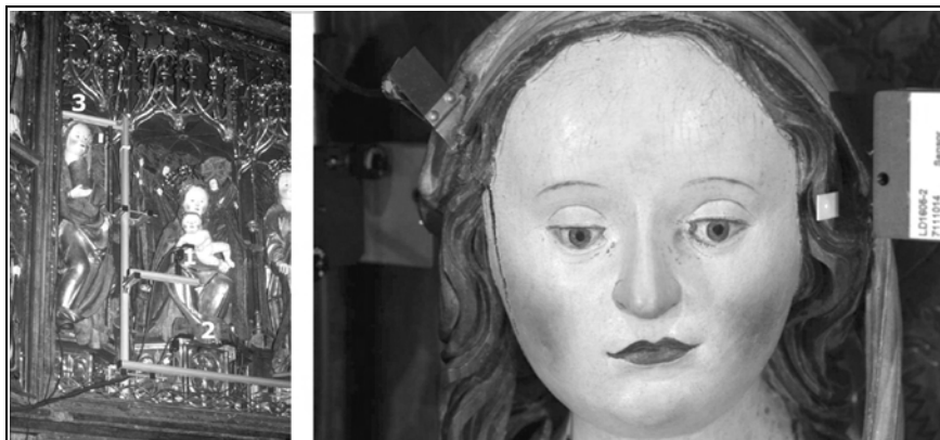
Figure 2.2. left: measurement set-up for measuring the dimensional changes of the wooden altar objects. Right: detailed view of measurement position 3, measuring the opening and closing of the crack in the head. (Photographs by Kozłowski / Kloda)
