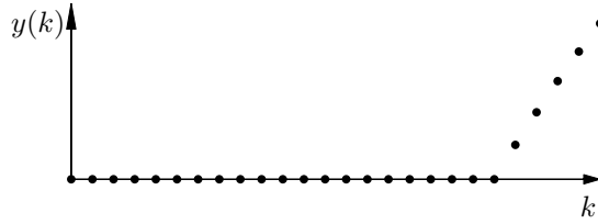
Fig. 3. Output of a system with a time delay of 20 samples.
