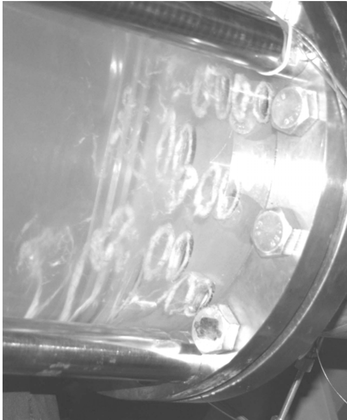
Figure 8 : Vortices visualization downstream a multi-hole orifice in lock-in regime (29)
