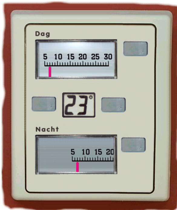
Figure 5.2: An inconsistent room thermostat. The daytime temperature control is implemented with a moving pointer and fixed scale, and the nighttime temperature control with a fixed marker and a moving scale. The daytime temperature is selected, which is indicated by the illumination.
