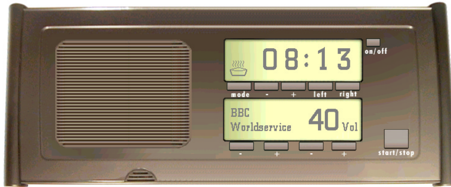
Figure 5.23: User interface of the radio alarm clock with a hot dish presented next to the timer time.
