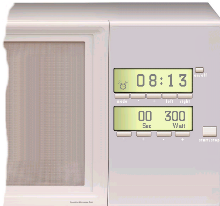
Figure 5.24: User interface of the microwave with a ringing mechanical alarm clock presented next to the timer time.
