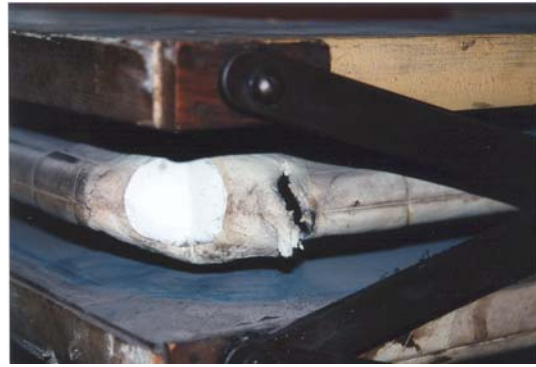
Figure 2. Damage to bellows
