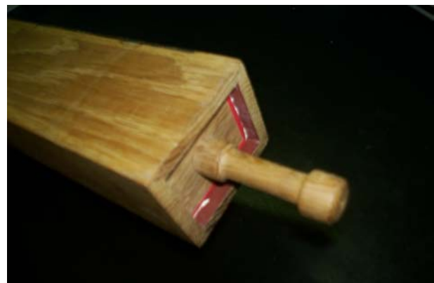
Figure 23. Wooden organ pipe with tuning cap
