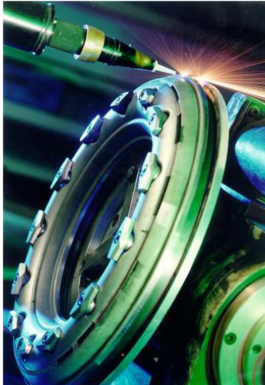
Figure 1.8: A photograph of a laser drilling process. (Courtesy Eldim B.V.)
