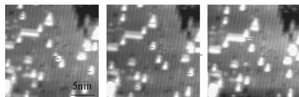
FIG. 2. Asymmetric scan of Sb on Si(001). These three scans were taken subsequently at 500 K after annealing the sample at 575 K. The tip is scanned at -2 V_{\text{substrate}} and 0.1 nA from left to right and then returned at -5 V_{\text{substrate}} and 0.3 nA from right to left. The bars indicate the position of a dimer which moved in the following frame. Here we find net movement of the free dimers along the tip sweep at high field.
