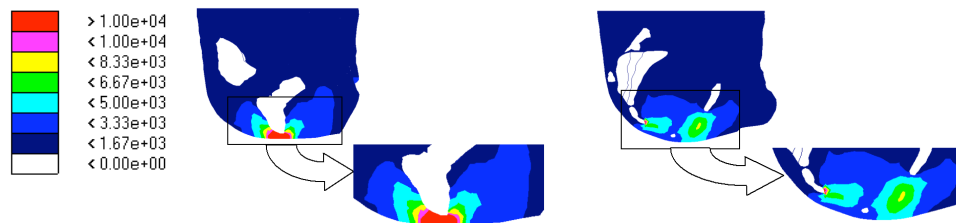
Figure 5.10: The von Mises stresses (Pa) in the soft tissues along a sagittal plane through the ischial tuberosities (left) and the coccyx (right) for a simulation with the FE buttocks model on a rigid surface.
