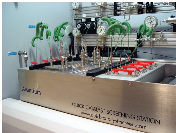
Figure 4-15. Reaction station with several blocks of twelve reactors connected to gas-inlet tubes.
