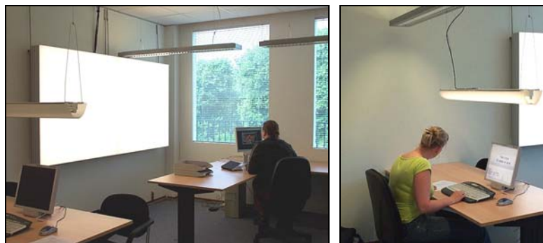
Figure 4.9: The test room with all different light sources used to create the variants: large luminous area (picture on the left), daylight (picture on the left), suspended luminaires (both pictures) and small luminous area (picture on the right)
