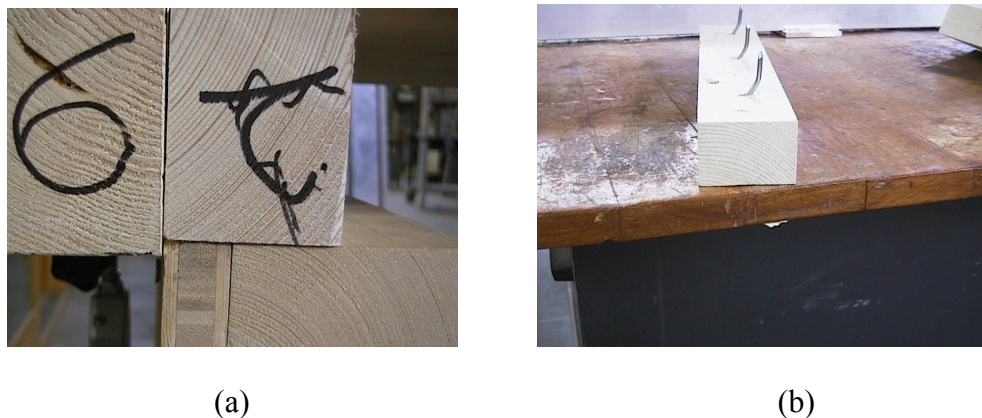
Figure 4-8 (a) SB1 test showing failure mode. (b) 75x50 wood piece removed from the left panel after the test showing how the nails were bent.
