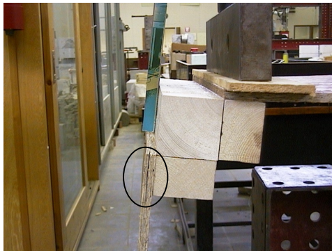
(b) First crack appears (delamination).
