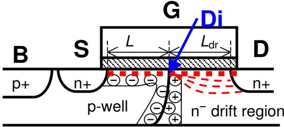
Figure 1. The SOI-LDMOS transistor
