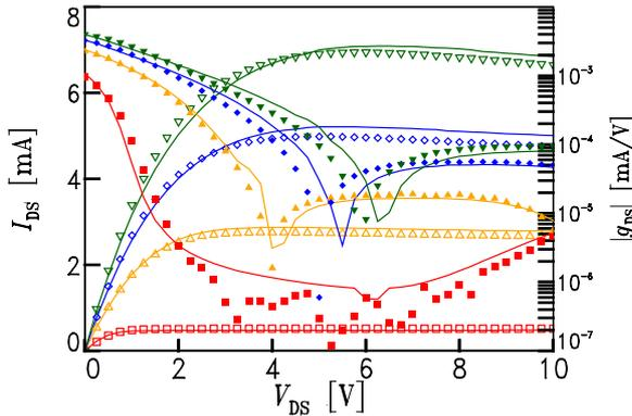
Figure 4. Drain current  $I_{DS}$  (open symbols) and output conductance  $g_{DS}$  (solid symbols) for  $V_{GS} = 3, 6, 9$  and  $12$  V, and  $V_{SB} = 0$  V.
