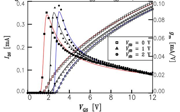
Figure 3. Drain current  $I_{DS}$  (open symbols) and transconductance  $g_m$  (solid symbols) in the linear operating regime, at  $V_{DS} = 0.1$  V.
