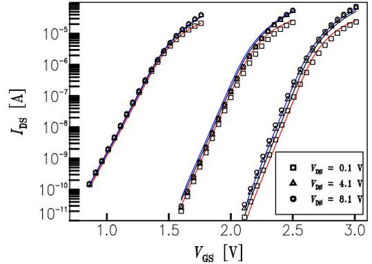
Figure 2. Drain current  $I_{DS}$  for  $V_{SB} = 0, 1$  and  $2$  V.
