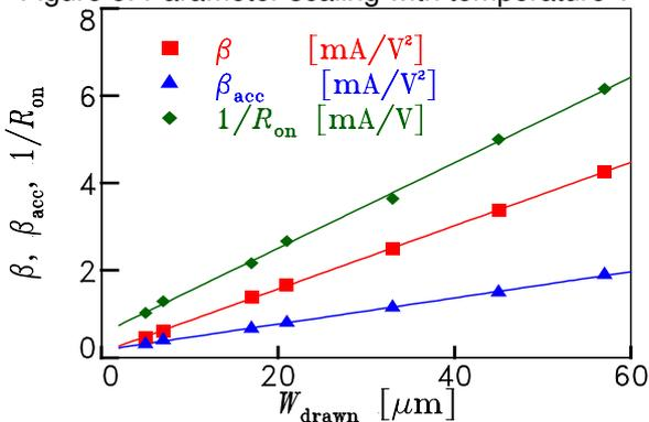
Figure 6. Parameter scaling with width  $W_{drawn}$ .
