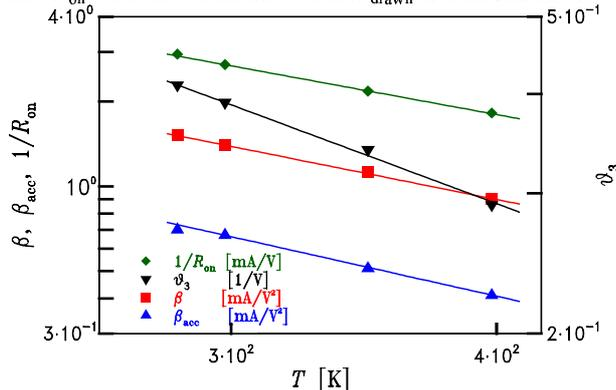
Figure 5. Parameter scaling with temperature  $T$
