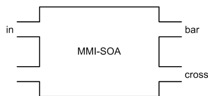
Figure 6.15: Schematic of the 2R-regenerator based on the 2 \times 2 MMI-SOA.
