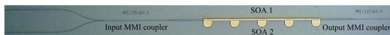
Figure 7.17: Photograph of the fabricated low-loss optical combiner with two simultaneously biased SOAs.
