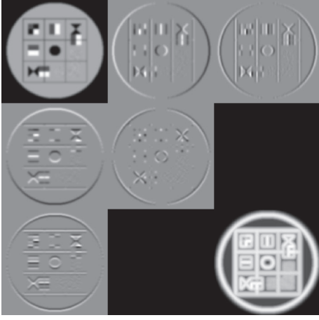
FIGURE 9: Hermite coefficients l_{n-m,m} , for m = 0, \dots, n , up to order n = 2 for a Gaussian window with spread \sigma = 2.5 times the sampling distance. The image in the lower-right corner is the residue amplitude A_r . To relate the mathematical results in this paper to the figures, it should be realized that the x -axis points to the right and the y -axis downwards. Moreover, the coefficients of order n , which are located in the n th diagonal, are amplified by the same factor \beta_n for display purposes. The factors \beta_n are chosen independently for each order n , in such a way that the complete display range is used.
