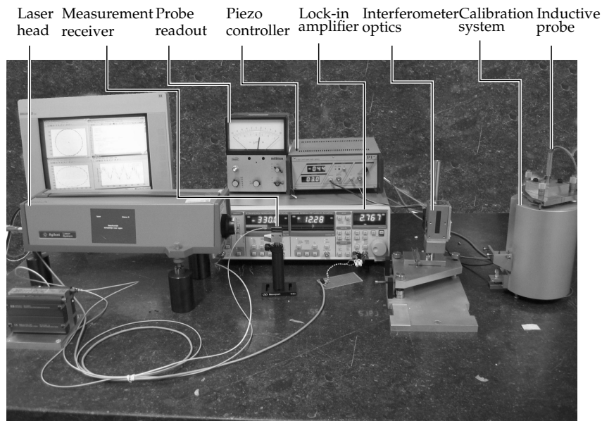
Figure 5.8: Photograph of the setup used to test the compensation method on a probe calibration setup.
