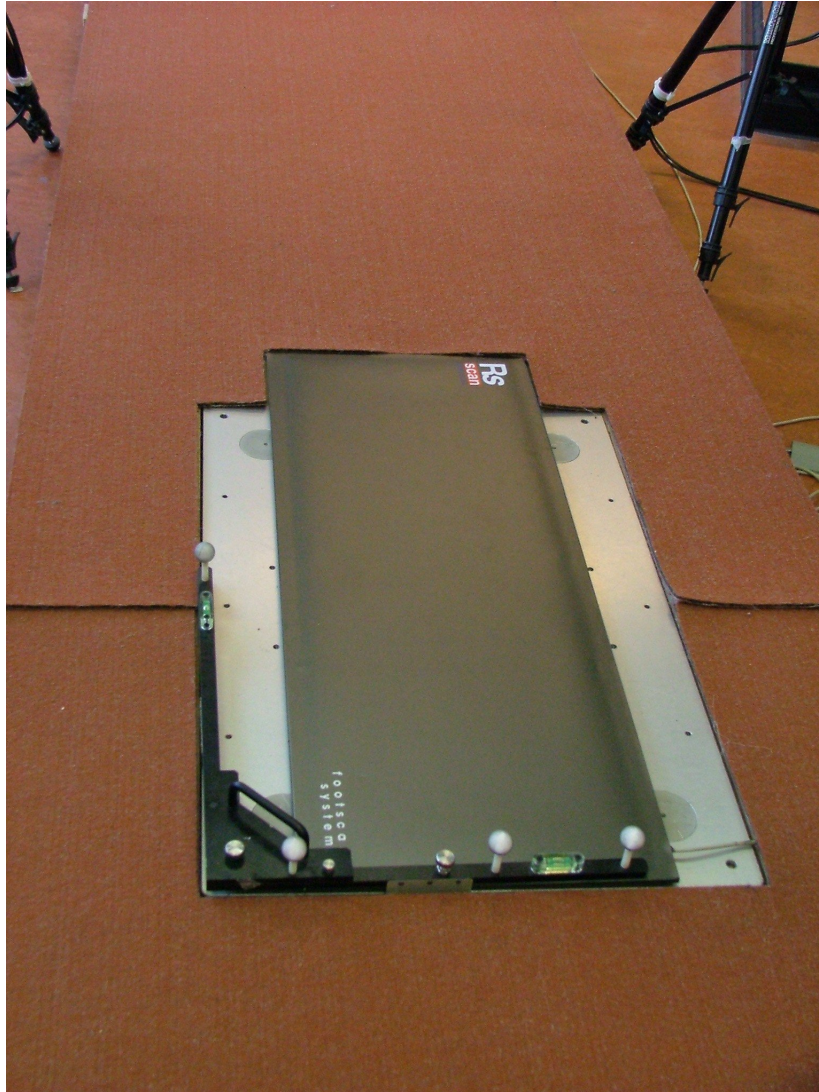
Figure 2.3 The coupled plate system. A one meter pressure plate is attached to a 90cm force plate. The L-frame in the left lower hand side is used to unify the local reference frames of the force plate and the motion analysis system.
