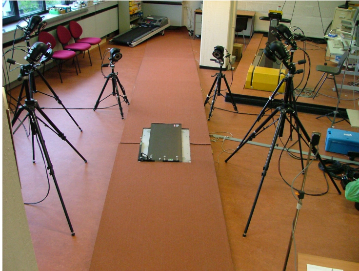
Figure 2.2 The camera set-up around the coupled plate system
