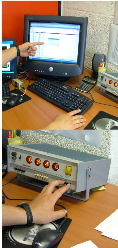
Figure B.4 Steps three and four of the dynamic registration tasks: above the preparation of MAS and below the resetting of the electronic timing device.
