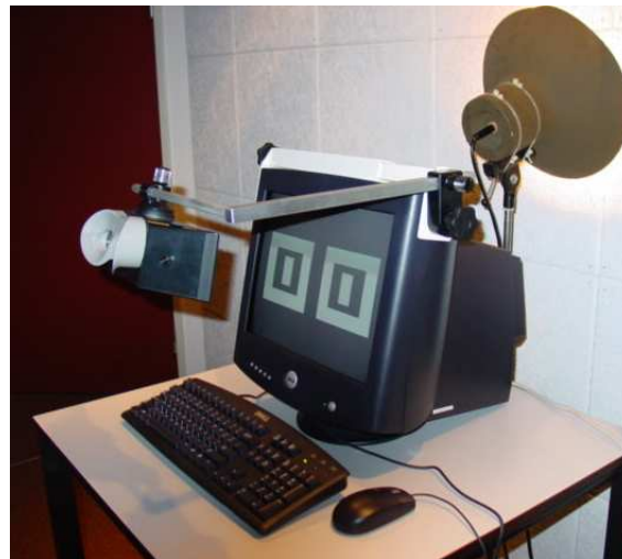
Figure 1.9: Screenscope™ attached to a PC monitor with a light source in the background. The monitor shows a stereoscopic test pattern illustrating the approximate size of the natural stimuli that were employed.
