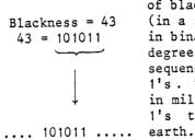
A picture is divided into little squares (pixels). For each pixel the degree of blackness is measured (in a scale of 0 - 63, in binary). So, this degree is described by a sequence of six 0's and 1's. The picture results in millions of 0's and 1's to be transmitted to
