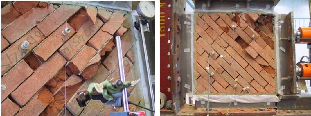
Figure 56 Remaining test pieces of thin layer mortar masonry after loading in two directions
