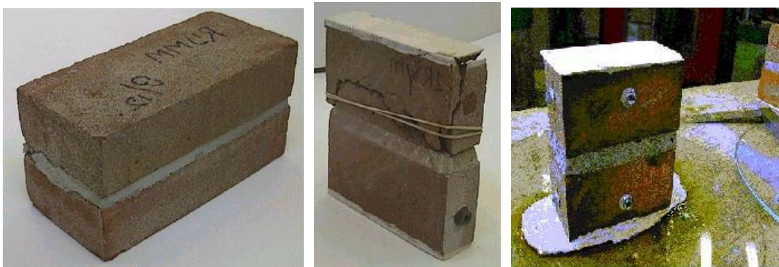
Figure 76 RW couplet, 25 mm thick specimen after testing, and capping of a specimen.
