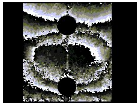
Figure 62 (left) Step 1 in the ESPI process: a speckle pattern image is obtained.
