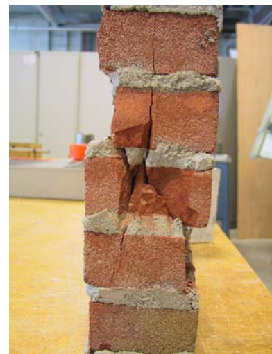
Figure 59 a) Phases in the failure process of a piece of masonry. b) Shear of a stack bonded specimen after spalling.
