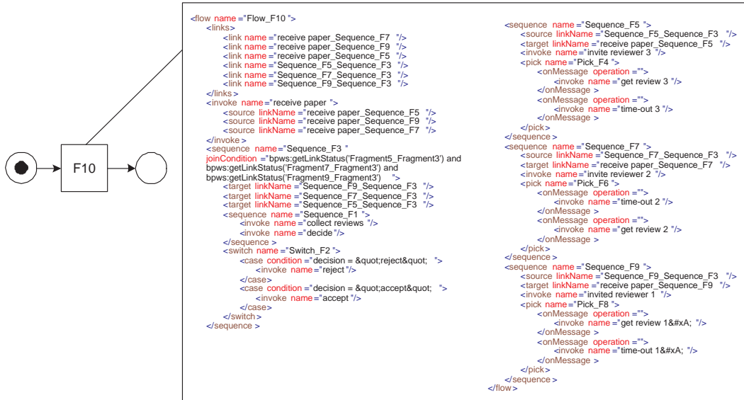
Fig. 7. The Petri net after replacing the remaining part by one transition F10 tagged with a flow expression.
