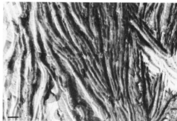
Figure 5. Electron micrographs of 1,4-t-PBD lamellae grown isothermally at 128 °C for (a) 5 min and (b) 120 min. Scale bar = 0.3 μm.
