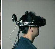
Figure 3.4: HMD based VR system: (a) A user in the immersive VR system; (b) HMD with head tracking sensor.
