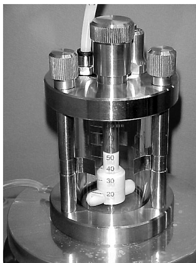
Figure 5.6: Picture of the ultrafiltration cell with pressure inlet (on top) and flow effluent (on bottom). Picture kindly provided by J. W. Weener.
