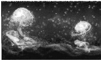
Figure 3.21: The creation of the quasi-spanwise vortex underneath the primary hairpin vortex for a droplet at Re_D = 1825 (side view, flow direction to the left). (a) the quasi-spanwise vortex is just created underneath the hairpin head (b) the flow at t = 0.1 s before the situation presented in photograph (a).
