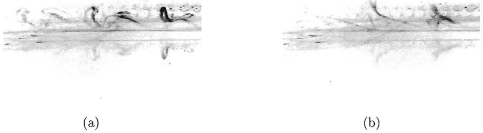
Figure 3.20: The vortex shape for Re_D = 1825 in the region 2 < x/D < 7 (side view, flow direction to the left). (a) droplet, (b) hemisphere.
