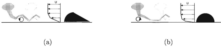
Figure 3.23: A schematic representation of the difference between the deformation of the legs for (a) a droplet (b) a hemisphere.
