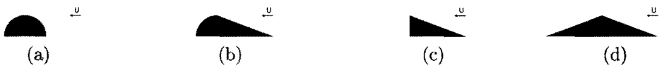
Figure 5.3: The four obstructions for which the shedding frequency was measured. (a) hemisphere, (b) droplet, (c) cone, (d) double cone.
