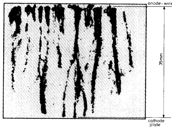
Fig. 5 Image intensifier picture, obtained with demagnification, showing emission of the discharge integrated in time ( V_p = 30 \text{ kV} )
