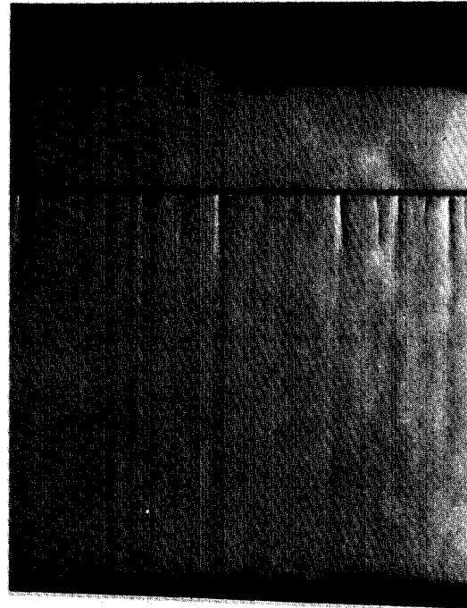
Fig. 10 Schlieren picture taken 100 \mu s after the start of the discharge ( V_p = 40 kV, gap distance = 50 mm)
