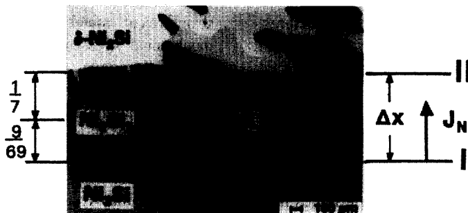
Fig. 1. Optical micrograph (polarized light) of a cross-section of a \delta\text{-Ni}_2\text{Si}/\text{Ni}_3\text{Si} diffusion couple annealed at 1043 K in vacuum for 70 h. Letter K indicates Kirkendall plane.
