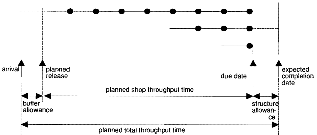
Figure 4.4: The three components of the planned total throughput time of an assembly order.
