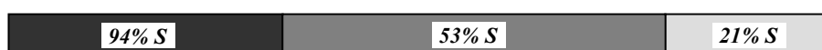
Scheme 6.1 Gradient copolymer of S and BA obtained in the three-step synthesis, schematically shown. The first block of M_n=1921 \text{ g}\cdot\text{mol}^{-1} contains 94% S, the second block of M_n=2610 \text{ g}\cdot\text{mol}^{-1} contains 53% S and the third block of M_n=1164 \text{ g}\cdot\text{mol}^{-1} contains 21% S.
